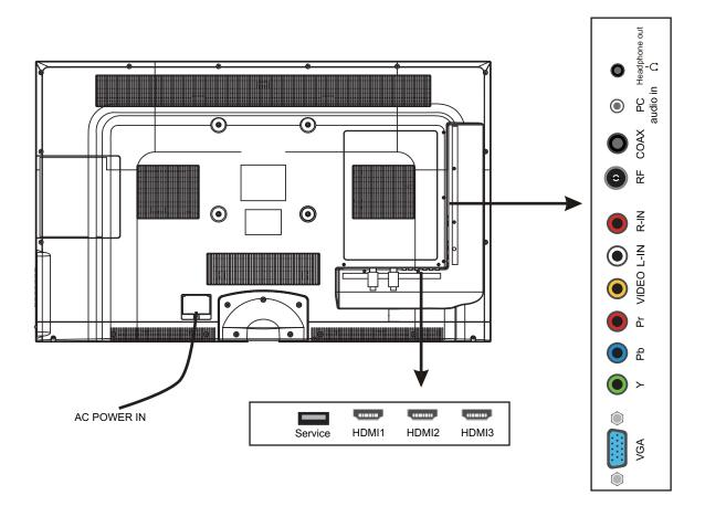
AC POWER IN: Connect to an earth 100-240V~ 50/60Hz outlet with the Power Cable.
